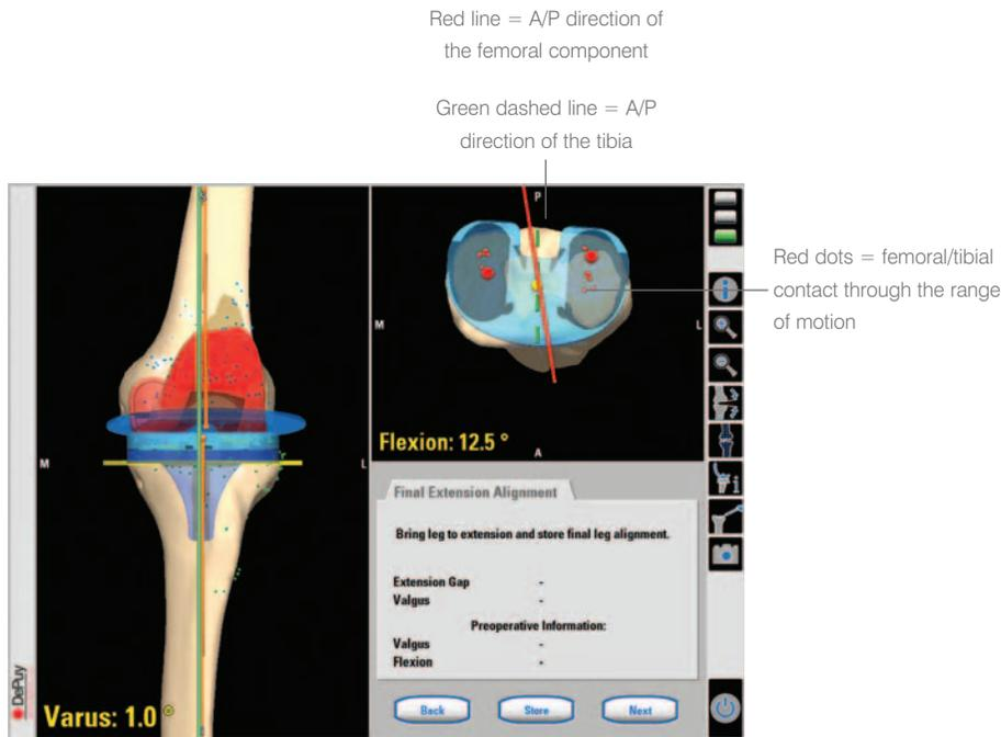
Motion analysis with trial components in extension
