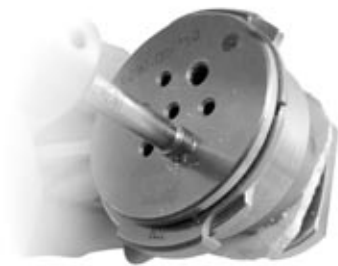
Step 4. Drill holes for the pegs
