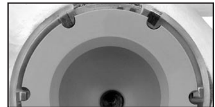
Anti-rotational tab and slot misaligned
