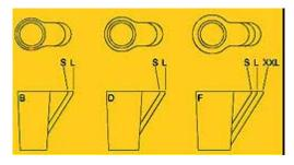
The final element that must be machined is the spout or triangle of the proximal sleeve. The triangle indicates the extension of the triangle from the outside diameter (O.D.) of the cone. Triangle sizing comes in Small, Large, or XX-Large.
