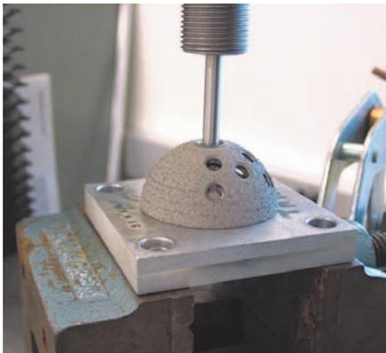
**Figure 3:** Push-Out test setup.
