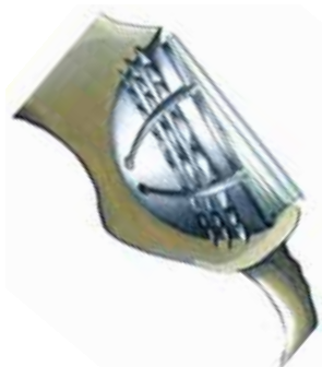
incorrectly positioned insert
