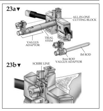
it seems that a larger offset might be needed, assess the fit of the next larger size femoral component. The change in stem position between sizes will help reduce the overall needed offset and prevent the component from being positioned too far posteriorly.
