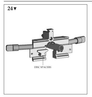
If a 5mm or 10mm Distal Femoral Augment is to be used, the corresponding spacer disc must be attached to the back of the All-In-One cutting block to insure the stability of the instrument (**Figure 24**).
