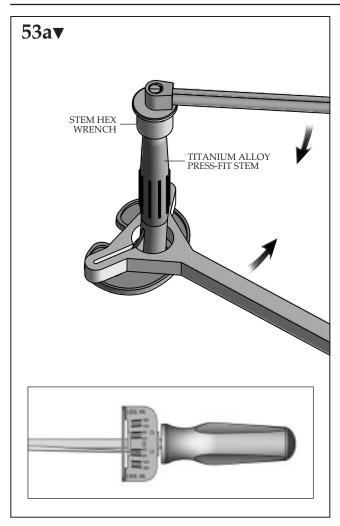
If a straight stem is used, remove the cap as stated previously. Tighten the stem extender into the tibial component by hand as far as possible. Attach the appropriate stem wrench to the torque wrench. Place the baseplate wrench on the tibial component. Holding the tibial component in your hand, engage the stem with the stem wrench and *tighten to 60in-lb minimum to 80in-lb maximum* (Figures 53a and 53b).
