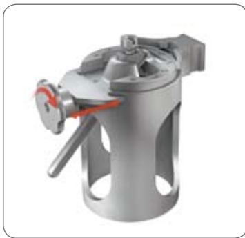
1. Mount the trial stem ball cylinder assembly into the impaction block and tighten the front slide to secure in place.
