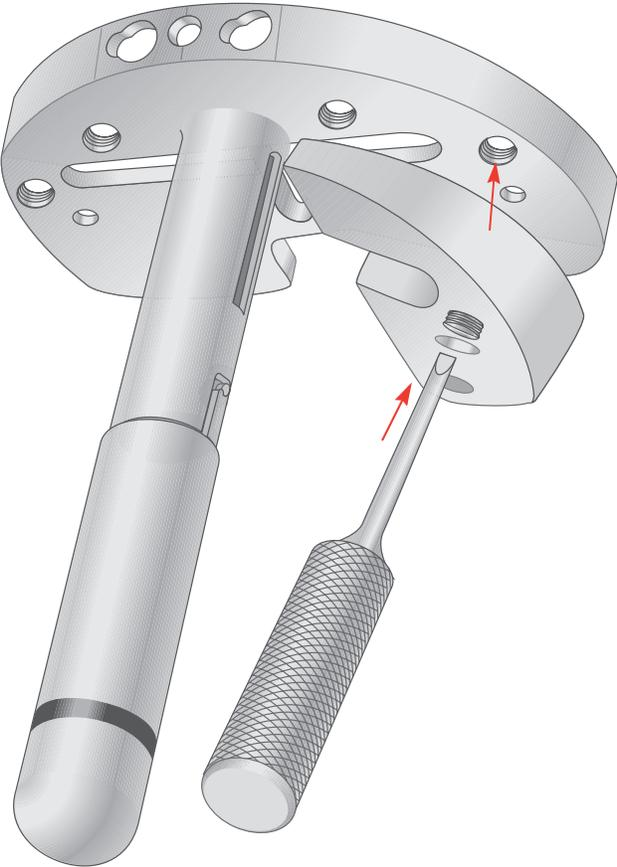
Positioning, alignment and security of the tray assembly is confirmed. If there is old cement or sclerotic bone present, relieve this first through the trial tray with a saw blade or burr prior to punching. The Specialist 2 tibial keel punch is appropriately positioned at the tray and cancellous bone interface and impacted into the keel configuration. The punch is carefully extracted and the tray assembly is subsequently withdrawn.
