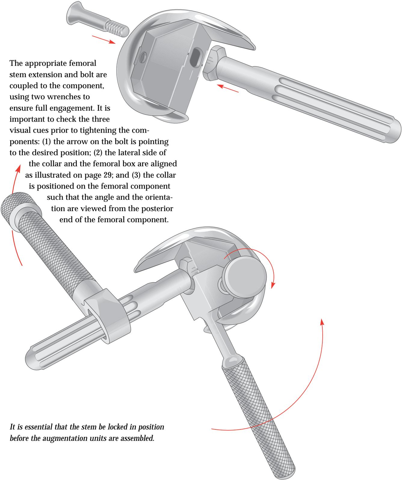
*It is essential that the stem be locked in position before the augmentation units are assembled.*
