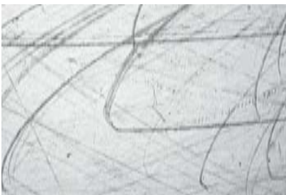
Surface of conventional polyethylene (6 months in vivo )
