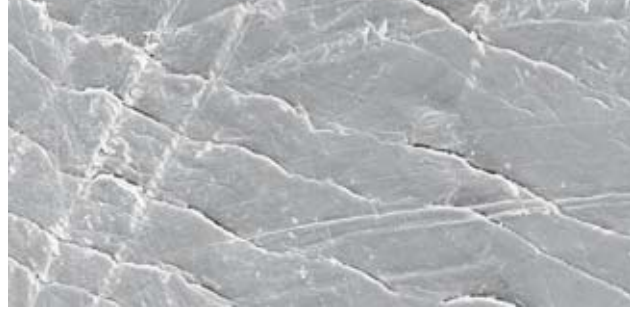
Ripples and overlaps on the Durasul explant
